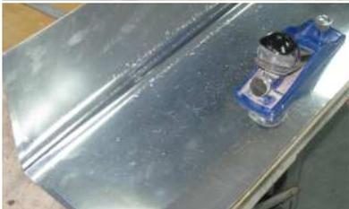
After trimming the aluminum to size, I break the edge, and use a block plane to get a straight smooth edge. That plane works great on Plexiglas too! I mark the nail locations, use an automatic center punch, then puncture the sheet for
