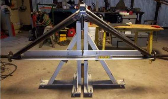
A veteran restorer is on the move also. **Jimmy Dean** is back to work on his Waco ASO project. One of the big challenges is about behind him...reconstructing the main gear... and getting the geometry just right...as in no more toe-in! Here is the gear in its custom made jig.
